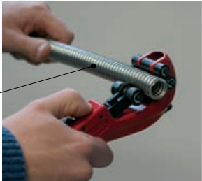
Exclusive 8-roller system for CSST corrugated pipe cutting easily and without pipe squeezing
