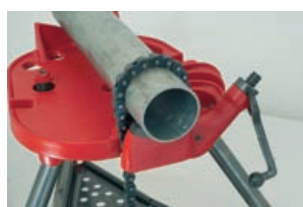
Example of chain pipe vice in the building site
